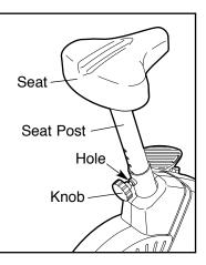
Next, slide the seat post up or down and align one of the adjustment holes in the seat post with the indicated hole in the Frame. Insert the knob into the frame and the seat post, and turn the knob clockwise until it is tight. Make sure that the knob is inserted through one of the adjustment holes in the seat post.
